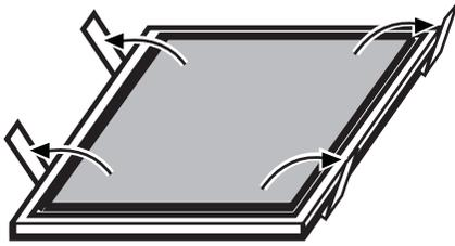
3. Place charcoal filter into top side of metal filter.
