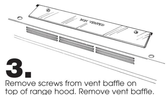
**3.** Remove screws from vent baffle on top of range hood. Remove vent baffle.
