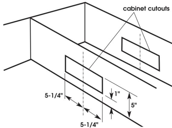
To vent through the roof with 3-1/4" x 10" rectangular vent, mark a line 1" and 5" from the back wall on the underside of the cabinet. Mark lines 5-1/4" to the right and left of the centerline on the underside of cabinet that connect the lines just drawn. Use a keyhole saw and saber saw to cut a rectangular opening for the ventwork. Repeat for the underside of the top of the cabinet.
