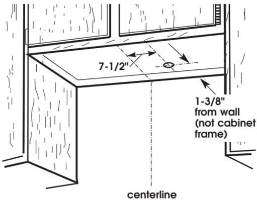
**9.** To wire through top, mark a line 7-1/2" from the right of the centerline on the underside of the cabinet. Mark the point on this line that is 1-3/8" from back wall. Drill a 1-1/4" diameter hole through the cabinet at this point. Note: If a cord-connection kit is used, drill a 1-5/8" diameter hole.
