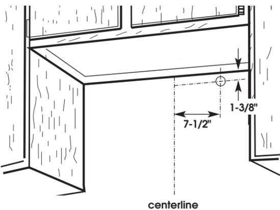
To wire through rear, mark a line 7-1/2" from the right of the centerline on the wall. Mark the point on this line that is 1-3/8" from underside of cabinet. Drill a 1-1/4" diameter hole through wall at this point.
