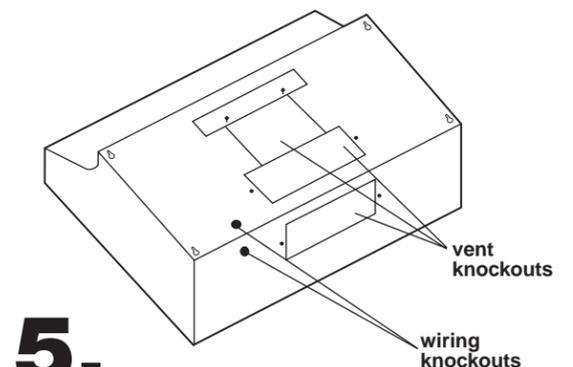
**5.** Remove knockout from the wiring opening (top or rear) to be used.
