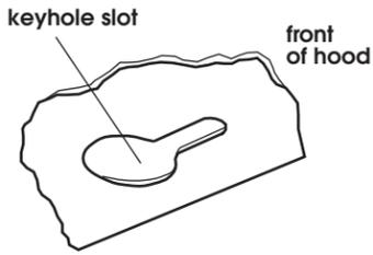
**7.** Lift the range hood into final position and center. Mark on the underside of cabinet the location of the four keyhole mounting slots. Set range hood aside on a protected surface.
