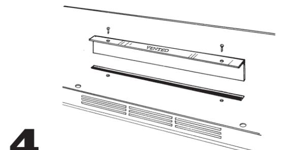
**4.** Turn vent baffle and reinsert in slot in top of range hood so that the word "Vented" is facing up. Fasten vent baffle with screws.
