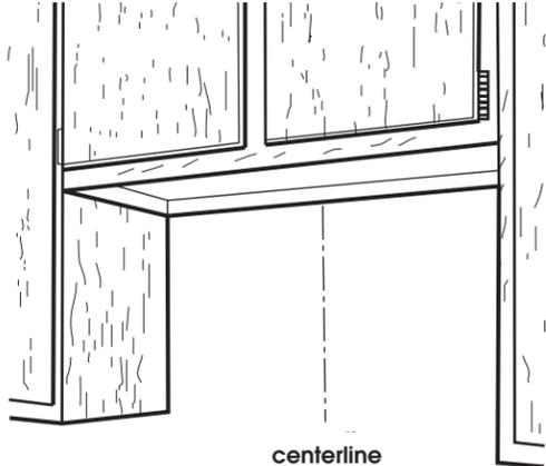
**8.** Determine and clearly mark a vertical centerline on the wall and cabinet in the area the vent opening will be made.
