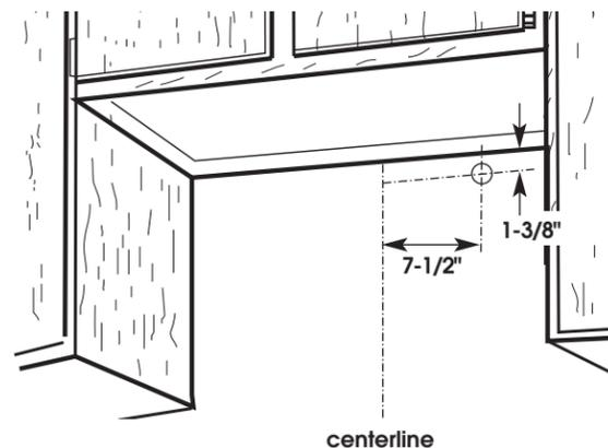
To wire through rear, mark a line 7-1/2" from the right of the centerline on the wall. Mark the point on this line that is 1-3/8" from underside of cabinet.
