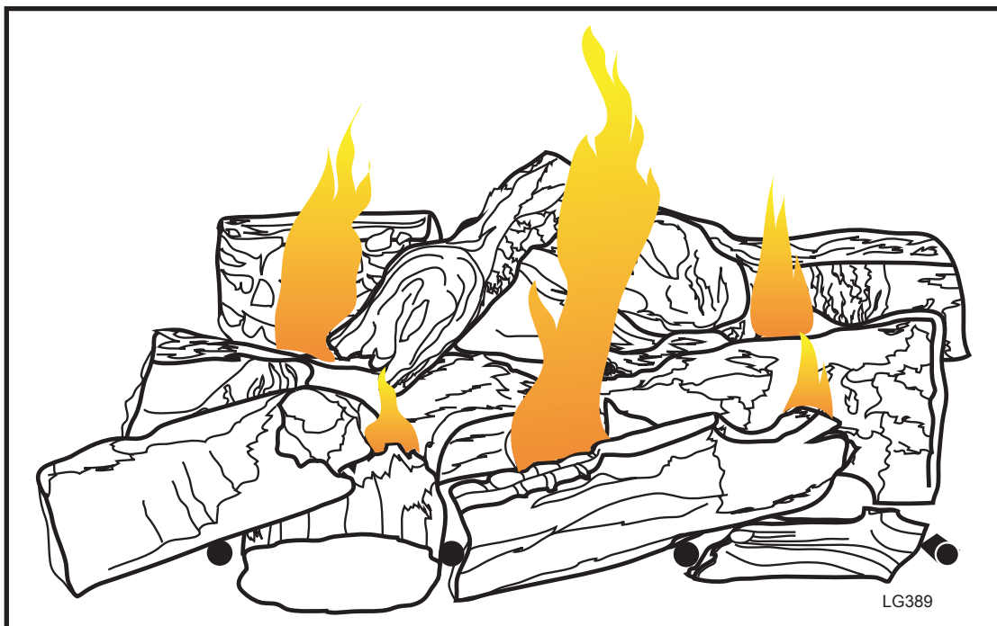
Fig. 57 Correct flame appearance for DVBR36 model.
