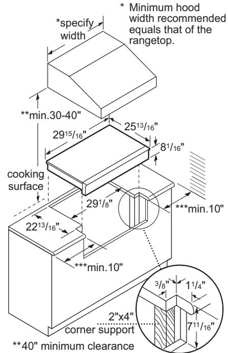
\*\*40" minimum clearance from cooking surface to combustible surfaces.
