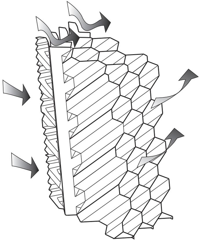
Integral drift eliminators prevent the costly nuisance of drift spotting on objects in the surrounding environment. Their unique shape induces the air flow through three distinct direction changes as illustrated above. The final turn directs air toward the fan to save you fan horsepower. Moisture carried in the air stream can't make these abrupt turns, so drift is 0.010% or less of the circulating water flow rate.
