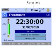
Ramp time is a feature that can be enabled by your clinician by setting a maximum ramp time. Designed to make the beginning of treatment more comfortable, ramp time is the period during which the pressure increases from a low start pressure to the treatment pressure. See "Setup menu: Options" on page 16.
