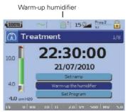
You can use the warm-up feature to pre-heat the water in the humidifier prior to starting treatment. The humidifier will be automatically detected when the device is turned on. The *Treatment* screen provides the option to start warming the humidifier. If the humidifier is heating, the related symbol is displayed at the top of the LCD screen.
