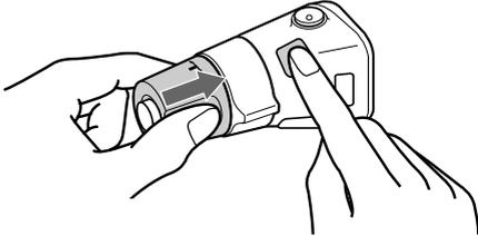
Press **(SOUND)** for two seconds while pushing the VOL control.
