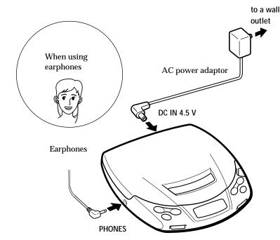
For models supplied with the AC plug adaptor If the AC power adaptor does not fit the wall outlet, use the AC plug adaptor.
