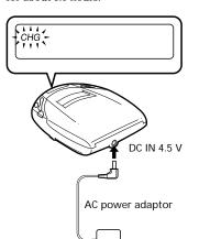
**4** When fully charged, "CHG" disappears. Disconnect the AC power adaptor.
