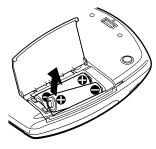
When to replace the dry batteries If the 🖾 indication appears in the display and the sound becomes inaudible, replace all the batteries with new ones, because the batteries become weak.
