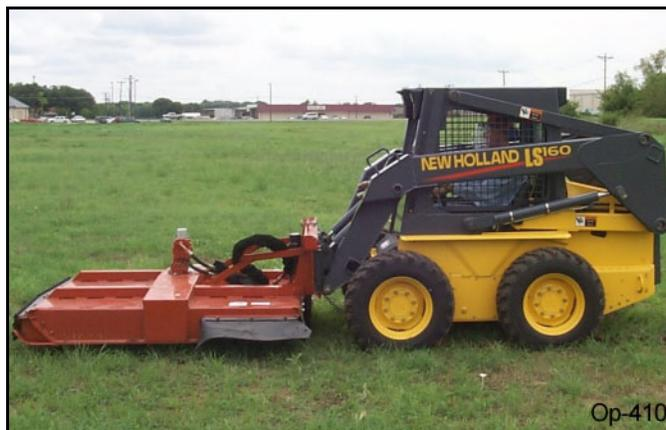
To avoid overturns, drive the skid steer with care and at safe speeds, especially when operating over rough ground, crossing ditches or slopes, and turning corners. Use extreme caution when operating on steep slopes. Travel at a slow speed when going downhill. DO NOT coast or free-wheel downhill.
