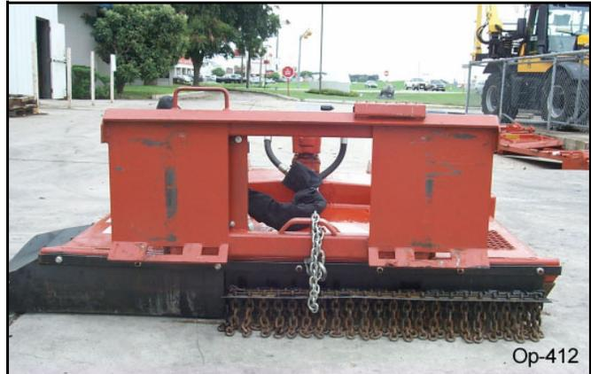
3. Remove the height limiting safety chain from the front of the skid steer chassis.
