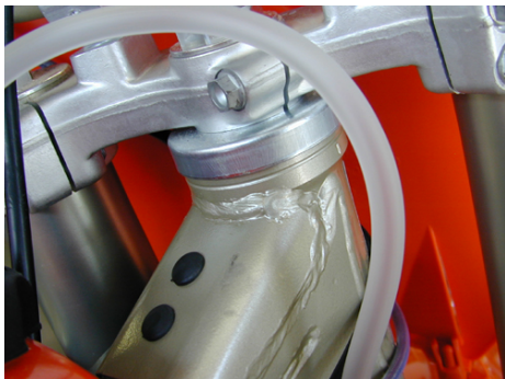
This example needs very little filing at the weld
