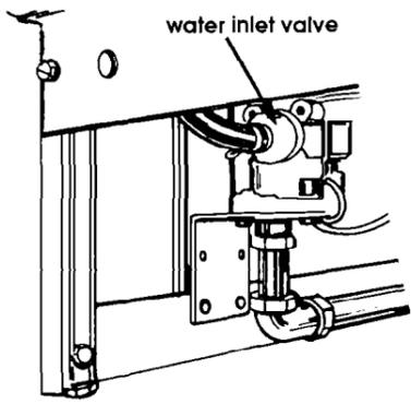
**10.** Connect water pipe or tubing directly to water inlet valve. Do Not run pipe or tubing across front of motor or dishwasher legs. Turn on water supply and check for leaks.
