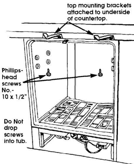
**12.** Open dishwasher door and remove all shipping materials. Remove bottom rack. Place a newspaper or large sheet of paper over bottom of dishwasher to protect the pump area when securing dishwasher to countertop.
