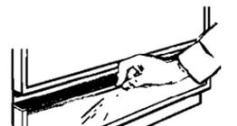
10. Insert wood access panel into access panel frame. Slide panel down into groove along bottom of access panel frame. It may be necessary to remove the two screws securing top of access panel to dishwasher frame and tilt access panel forward to install some wood panels.
