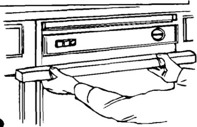
**8.** Latch dishwasher door. Push dishwasher into place, sliding drain hose through hole cut in cabinet opening. **Do not pinch power supply cord or kink power supply cable between dishwasher and cabinet.** Check that front leveling legs are firmly against the floor. Align dishwasher door with cabinet doors, so that spacing is the same on both sides.
