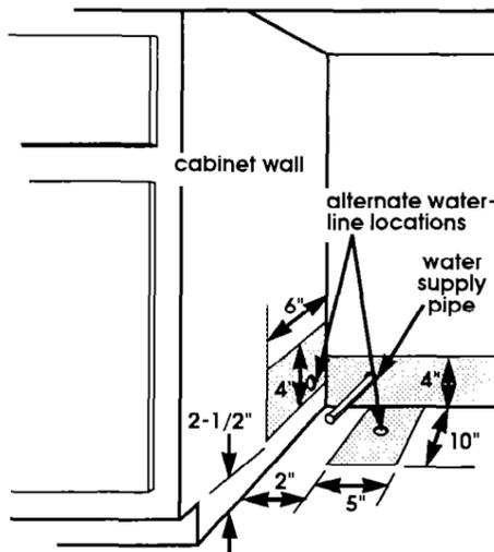
**1.** Rough in water line to the dishwasher cabinet opening using one of the routing methods shown. Cut 1/2" or larger hole in cabinet wall for water line.
