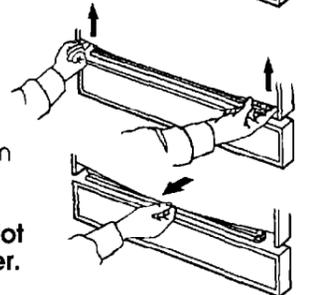
**3.** Insert one side of door panel(s), with desired color facing out, into one side of door frame.
