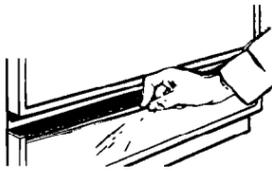
3. With desired color facing out, bow access panel and insert into access panel frame. Slide panel into groove along bottom of access panel frame.
