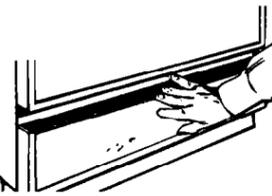
4. Line up edges of top trim with sides of access panel frame. Tilt back of trim down and slide into place. Snap front of trim down to cover top edge of access panel.
