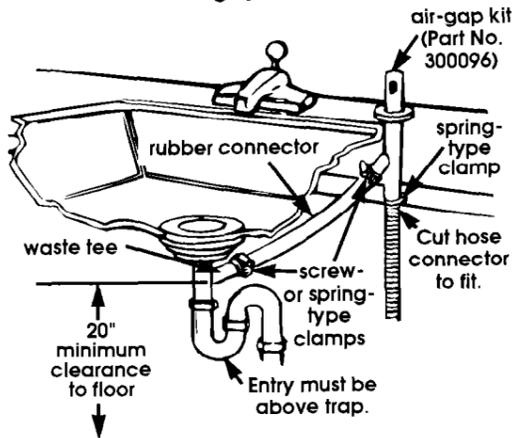
Drain hose to air gap to disposer.
