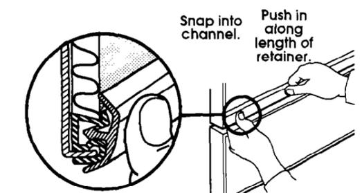
**6.** Snap one end of retainer into channel as shown. Push inward while sliding thumb along full length of retainer.
