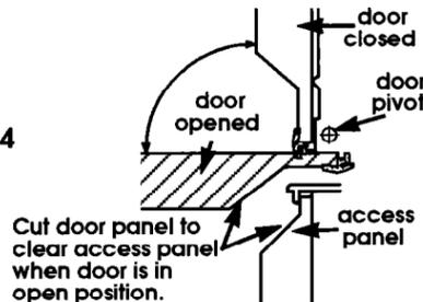
Heavy-duty door springs must be used if custom door panel weighs more than 4 pounds. Heavy-duty Door Springs Kit, Part No. 4318050, is available from your dealer or parts supplier. Maximum door weight is 8 pounds.
