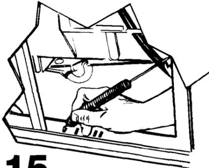
**15.** Check door for proper operation. Door should close easily without slamming and open with its own weight. If necessary, close door and adjust both door springs by moving spring ends to different holes in base.
