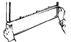
9. Carefully slide color access panel and spacer upwards and remove. Save color access panel and spacer for future use.
