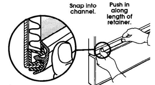
6. Snap one end of retainer into channel as shown. Push inward while sliding thumb along full length of retainer.
