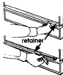
4. Lift door panel(s) at outer edges. Use one hand to bow bottom of panel(s). Remove panel(s) and spacer. Save panel(s) and spacer for future use.
