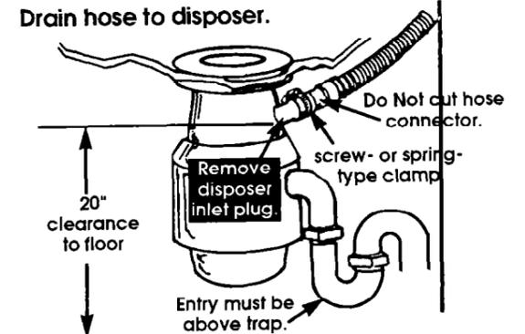
If local plumbing codes permit, dishwasher drain hose may be connected directly to disposer. Most disposers have 7/8" connectors or special connectors are available at plumbing supply houses.
