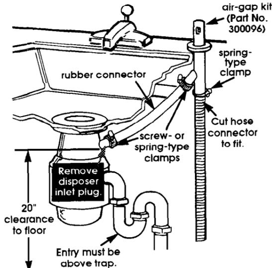
Install air gap (Part No. 300096)\* according to kit instructions. If other brands of air gaps are used, they should be checked to make sure they allow for the same water flow.
