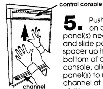
**5.** Push in on door panel(s) near the top and slide panel(s) and spacer up inside bottom of control console, allowing panel(s) to rest on channel at bottom of doors.
