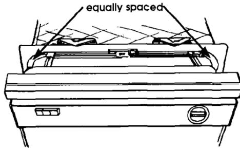
**14.** Open door approximately 3" and check for equal spacing between inner door and tub sides. If necessary, loosen screws that fasten dishwasher to countertop and shift tub. Tighten screws.
