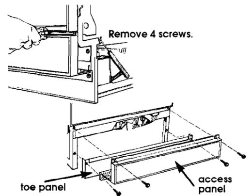
**5.** Remove the 4 screws attaching access panel and toe panel to dishwasher using a 1/4" hex socket, nut driver or Phillips screwdriver. Remove access panel and toe panel.
