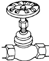
**3.** Flush water line into a bucket to get rid of any particles that may clog inlet valve. Turn shutoff valve to the "OFF" position.
