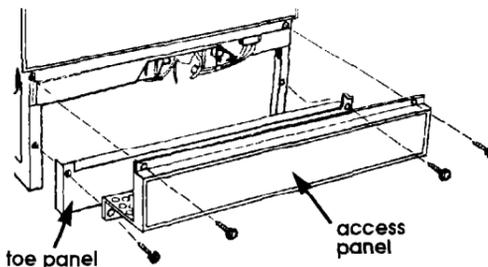
**19.** Replace the access panel and toe panel. The toe panel must be positioned to contact floor.
