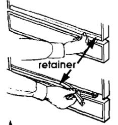
**2.** Lift door panel(s) at outer edges. Use one hand to bow bottom of panel(s). Remove panel(s). Do Not remove spacer.
