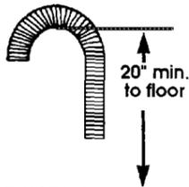
**NOTE: An air gap MUST BE USED in the high drain loop if the drain hose is connected to house plumbing lower than 20" above the floor.**
