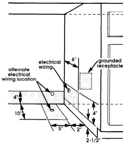
**4.** Cut a 1-1/2" maximum hole for power supply cord or a 3/4" minimum hole for direct wiring in the cabinet or floor for the electrical wiring to pass through. If this hole is cut in a wood cabinet, sand the hole until it is smooth. If the hole is cut in a metal cabinet, the hole **must** be covered by a grommet (Part No. 302797), available from your dealer or parts supplier.
