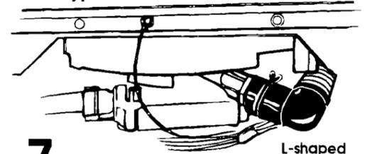
**7.** Put spring-type drain hose clamp over connector. Push drain hose onto connector. Use pliers to open clamp and slide clamp over drain hose and connector. Check that drain hose is secure.
