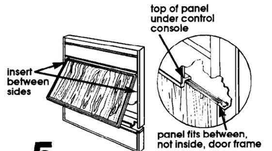
5. Insert top of wood door panel between sides of door frame about 3" below console. Rotate wood door panel down against dishwasher door. Slide top edge of wood door panel under bottom edge of console. Press lower portion of wood door panel in place between sides of door frame, allowing wood door panel to rest on channel at bottom of door.
