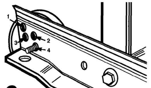
**6.** Measure height of cabinet opening from the front edge of the underside of cabinet opening to floor. Check chart for that height opening. Put the wheels in the required position. The dishwasher should be installed as level as possible from front to back.
