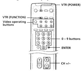
Use the video operating buttons on the remote commander to operate the video equipment. Press VTR (FUNCTION) before operating the video equipment.
