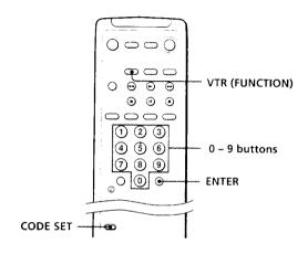
Press the CODE SET, VTR (FUNCTION), and 0 – 9 buttons to enter the manufacturer's code number (see the chart in the following page), then press ENTER. For example, to operate a Sony 8 mm VCR, press CODE SET, VTR (FUNCTION), 3, 0, 2, and ENTER.
