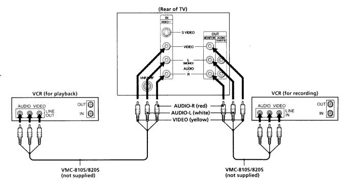
The above type of connection should only be used when you connect from the line input of one VCR, and from the line output of a second VCR.
