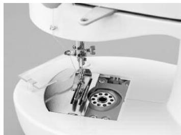
The machine may have come pre-threaded from the factory. Look at this threading carefully before removing it to replace the thread or bobbin with different thread. Then follow the preceding instructions to rethread.
