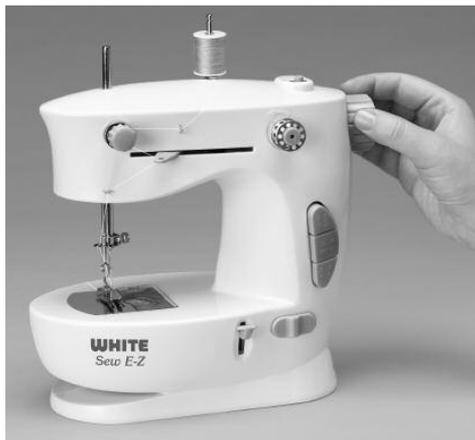
Rotate the handwheel to bring the needle to the highest position.
