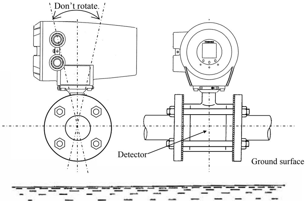
**Figure 4.6 Installation position of the detector**
