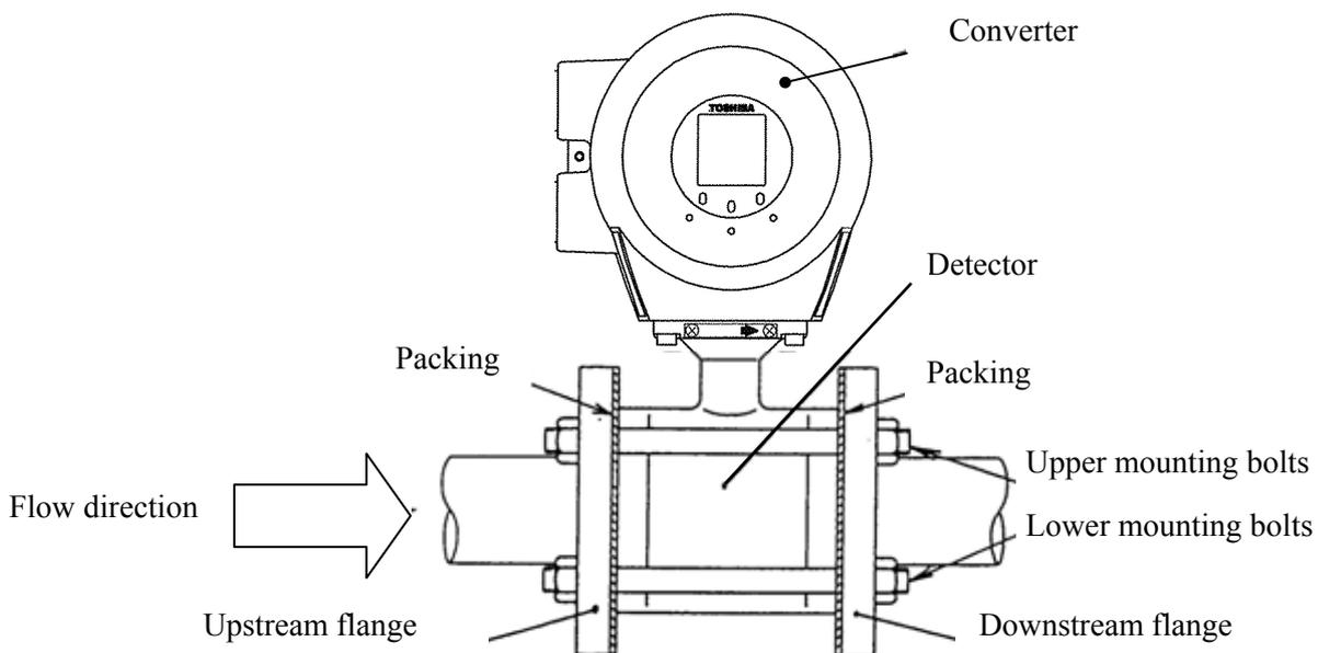
Figure 4.4 LF516/LF546 flowmeter piping connections
