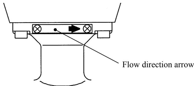
**Figure 4.7 Flow direction arrow on the detector**
