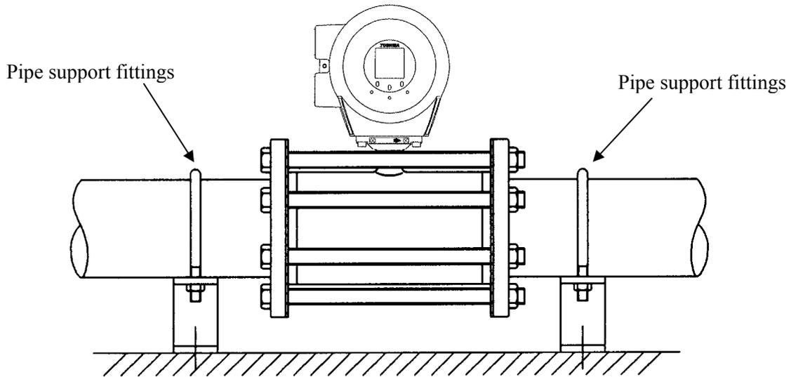
Figure 4.2 Example of Pipe Fixing Procedure
