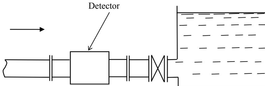
**Figure 4.9 Detector with sufficient head pressure at downstream outlet**
