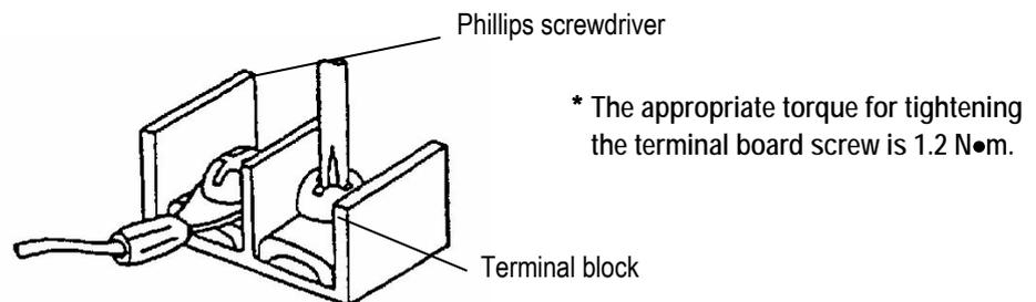
**Figure 5.10 Connecting a Cable to Terminal Block**
