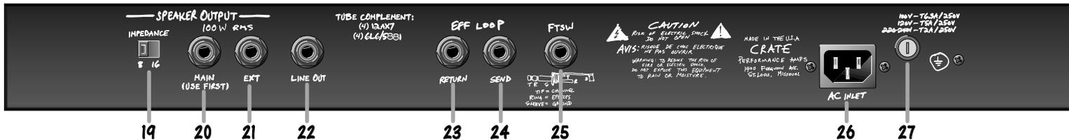
**19. IMPEDANCE SELECTOR:** For the best performance and least strain on your amplifier, you **MUST** properly match the impedance of your amplifier to that of your speaker cabinet(s). Set the selector switch to the 8 or 16 ohm position, depending on the **total** impedance of your speaker cabinet(s). The chart below can help you determine that impedance based on the following combinations of speakers connected in parallel.
