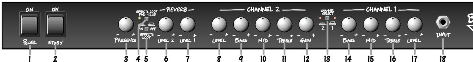
**1. POWER:** This switch applies AC voltage to the amplifier, and should always be turned **on first**. The switch illuminates when the AC power is on.
