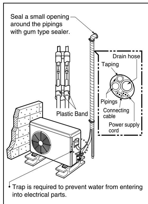
In case of the Outdoor Unit being installed above position of the Indoor Unit.
