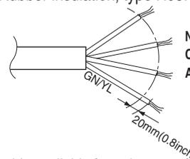
**NORMAL CROSS-SECTIONAL AREA 2.1mm<sup>2</sup> (AWG 14)(24k/34k)**
