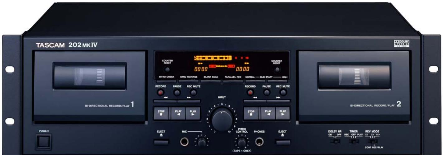
The TASCAM 202mkIV is a 3U rack-mountable dual cassette deck with the ability to record on one-or-both wells of the deck. The cassette deck includes Dual Auto Reverse, 12% +/- Pitch Control on Tape Deck 1, and Power on Play and Record. The unit is equipped with a front panel Microphone Input with level control, Dolby B noise reduction, and a Headphone output.
