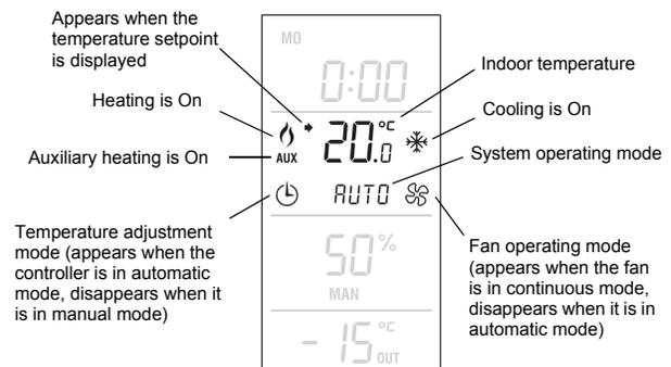
The controller normally displays the measured indoor temperature. To view the setpoint, press one of the **▲▼** buttons. The setpoint will be displayed along with the symbol for the next 5 seconds.
