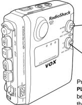
Set REC SPEED to NORM for normal recording or to EXT for extended recording (twice the normal recording time). When **REC SPEED** is set to **EXT**, the recorder puts the recording in half the space used during normal speed.
