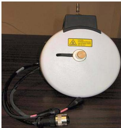
**Figure 15** Multimode Spray Chamber
