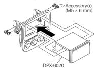
2 Install the center panel with the unit in your car.
