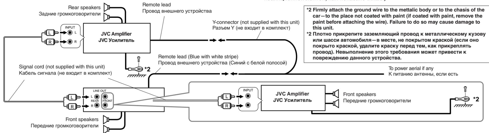
\*2 Firmly attach the ground wire to the metallic body or to the chassis of the car—to the place not coated with paint (if coated with paint, remove the paint before attaching the wire). Failure to do so may cause damage to this unit.
