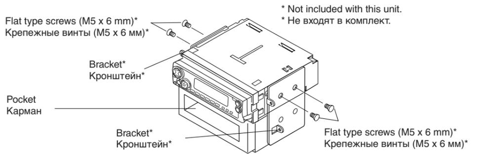
**Note:** When installing the unit on the mounting bracket, make sure to use the 6 mm-long screws. If longer screws are used, they could damage the unit.
