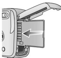
3. To close, push the battery chamber cover until you hear a click. If the memory card does not slide in smoothly, do not attempt to insert it by force. Check the direction of insertion, and then insert it correctly. Do not insert the memory card the wrong way round. Doing so may damage the memory card slot.
