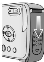
2. Have the front of the memory card facing toward the front of the camera (lens) and the card pins toward the back of the camera (LCD monitor), and then push the memory card into the card slot until you hear a click.
