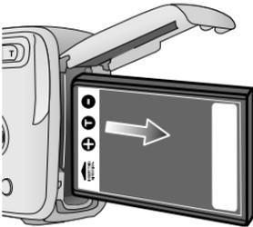
1. Turn off the camera power. Open the battery chamber cover and move the battery holder aside. The battery will be released.
