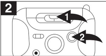
Push the PLAY button ❶ to start playback and adjust the VOLUME control ❷ as desired.
