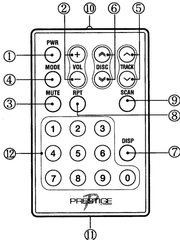
The wireless remote control supplied with this model is capable of operating many of the features of the unit as well as some additional ones from a remote location. Each button on the remote control functions in the same way as the referenced button on the main unit. For optimal operation of the remote control, always aim it toward the Remote Sensor ②⑥ on the front panel of the main unit.
