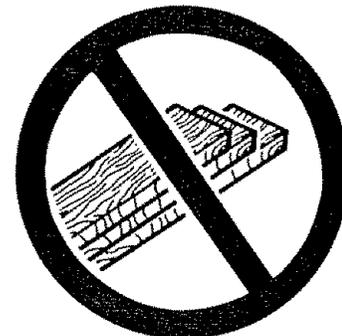
3. Rip only workpieces longer than the diameter of the blade. Do not rip workpieces that are shorter than the diameter of the blade being used.
