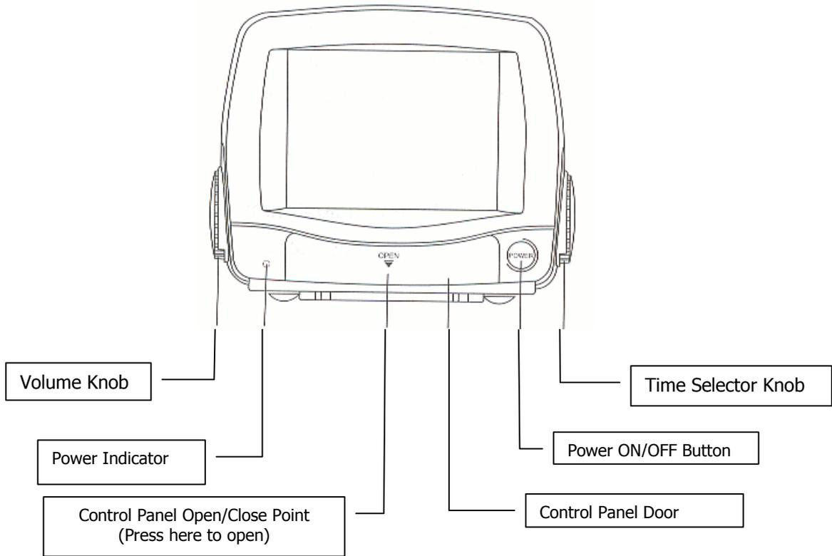
**With the control panel open, the following items are in view:**
