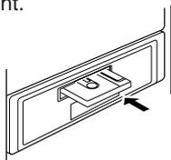
When the cassette is loaded, the player automatically starts tape playback and indicates "TAPE" in the display.
