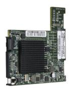
High performance computing (HPC) solutions have used InfiniBand networks to meet the needs of the most demanding set of applications and grand challenges. The QME7342 is a dual-port, 40Gbps InfiniBand-to-PCI Express® Gen2 x8 Host Channel Adapter designed for the Dell® PowerEdge® Blade Server. The QME7342's highly integrated design delivers unprecedented levels of performance, making it the ideal solution for HPC applications that rely on low latency, direct-memory access.
