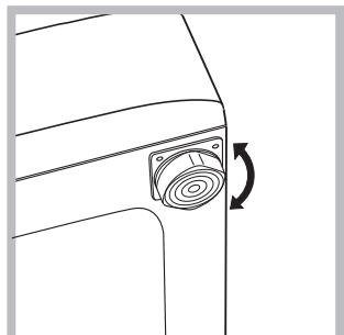
2. If the floor is not perfectly level, compensate for any unevenness by tightening or loosening the adjustable front feet (see figure); the angle of inclination, measured in relation to the worktop, must not exceed 2°.
