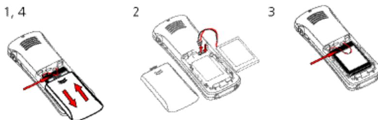
*Figure 10 Battery replacement*
