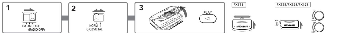
**1** Set FM/AM/TAPE (RADIO OFF) to TAPE (RADIO OFF).
