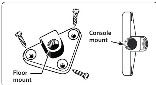
Step 2. Using the base as a template, drill three 1/8" holes and attach base with the included self-tapping screws. Snap screw caps in place over the screws on the base.
