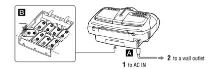
Connect the AC power cord **A** or insert eight R20 (size D) batteries (not supplied) into the battery compartment **B**.
