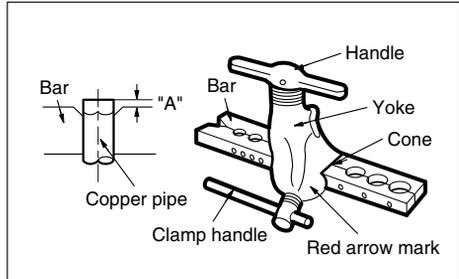
Firmly hold copper tube in a bar(or die) as indicated dimension in the table above.
