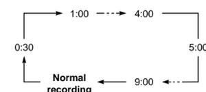
The tape counter decreases minute by minute to 0:00, then the unit stops recording and turns off automatically.
