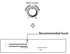
The bias current is now properly adjusted and the tape sensitivity compensation has been set. Press ■, then press CALIBRATION to turn the calibration function off (the display returns to normal). Rewind the tape and start the actual recording.
