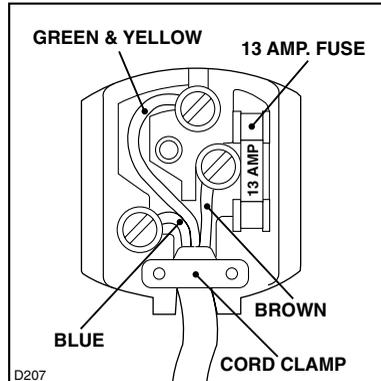
Connect the Green and Yellow (earth) wire to the terminal in the plug which is marked with the letter «E» or the earth symbol
