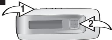
Press the MENU/Lock button **1**; the Main menu will appear. Scroll to Settings by pushing the Navigation control towards **◀** or **▶** **2**, then press the Navigation control **2**.
