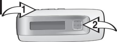
Press the MENU/Lock button **1**; the Main menu will appear. Scroll to Settings by pushing the Navigation control towards **◀** or **▶** **2**, then press the Navigation control **2**.
