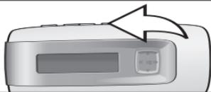
Turn the unit on by pressing the Power On/Off/Stop button; the Memorex start screen will appear in the display temporarily. Then the Music Player menu will appear and the MP3/WMA's track information will appear in the display.
