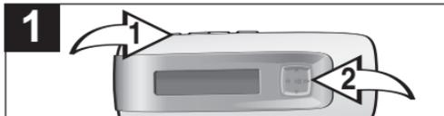
While in FM Playback mode, and with a desired station selected, press the Menu/Lock button ❶; the FM Menu will appear. Push the Navigation control towards ▲ or ▼ ❷ to select Add to Preset, then press the Navigation control ❷.
