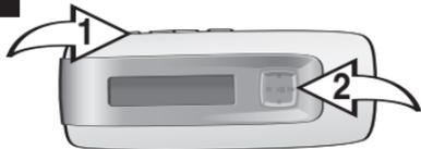
Press the MENU/Lock button **Ⓜ**; the Main menu will appear. Scroll to Settings by pushing the Navigation control towards **◀** or **▶** **Ⓝ**, then press the Navigation control **Ⓝ**.
