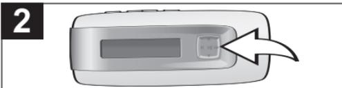
Push the Navigation control towards **▲** or **▼** to select the Preset station which you want to delete and press the Navigation control. Select YES (delete the Preset) or NO (cancel deleting the Preset) by pushing the Navigation control towards **◀** or **▶**, then press the Navigation control.
