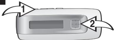
Press the MENU/Lock button ❶; the Main menu will appear. Scroll to Settings by pushing the Navigation control towards ◀ or ▶ ❷, then press the Navigation control ❸.
