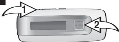
Press the MENU/Lock button ❶; the Main menu will appear. Scroll to Settings by pushing the Navigation control towards ◀ or ▶ ❷, then press the Navigation control ❷.
