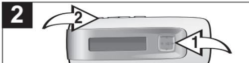
Select a desired Preset by pushing the Navigation control towards ▲ or ▼ ❶, then press the Navigation control ❶ to add the station to the Preset. To exit the FM Menu, press the Menu/Lock button ❷ twice.
