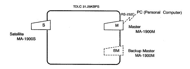
This system can be configured as one of the following two system types. The number of MA-1900 ECR units that can be connected in each system is indicated below.
