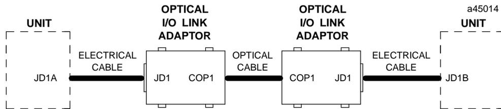
Connection between a master or slave device and an Optical Adapter is made using electrical cable A03B-0807-K803, which is a one-meter cable with connectors on both ends. Connect this cable to JD1 on the adapter. A connection diagram is shown below.
