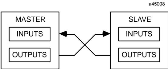
For each Series 90-70 I/O Link Interface Module used as a master, %I and %Q references and data lengths for each slave are assigned within the application Program Block, using Logicmaster 90. Instructions for doing this are given in chapter 4. For other types of devices on the link, references and data lengths are assigned differently. For details on how a specific type of device handles its I/O Link data, you should refer to the User's Manual for that device.
