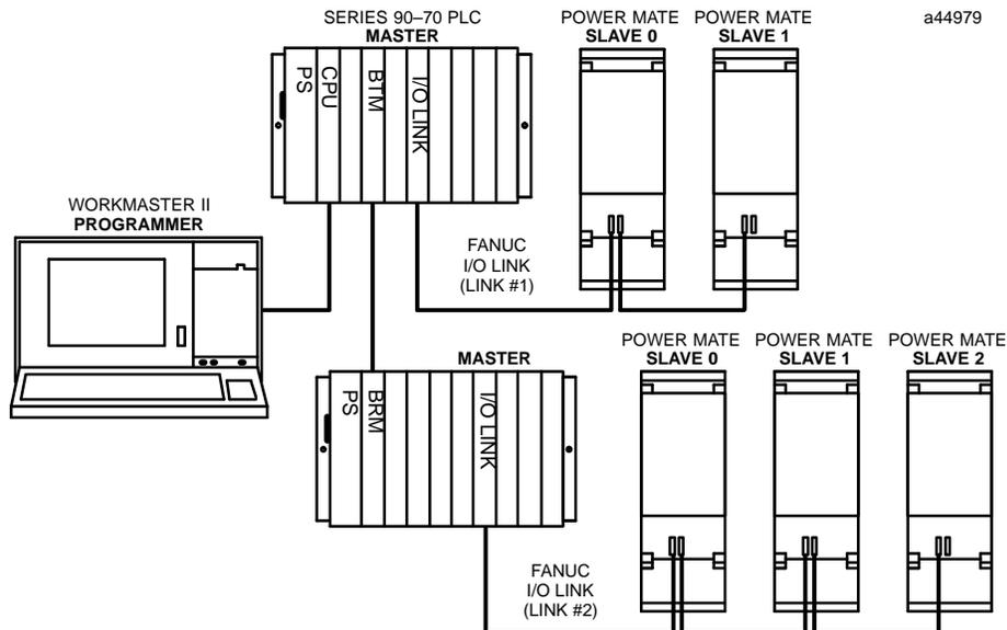
Up to four I/O Link Interface Modules can be installed in a Series 90-70 PLC. They can be located in the CPU rack and in expansion racks. Each I/O Link Interface Module can be used in either master or slave mode.
