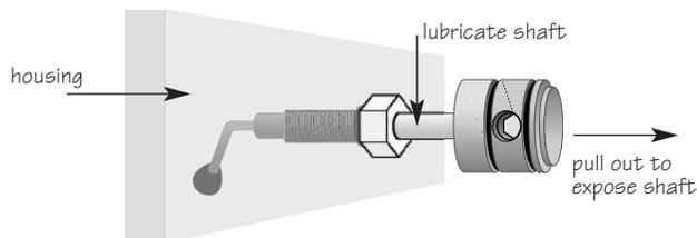
pulled out, exposing the shaft (see drawing).
