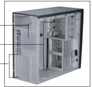
Rear 120mm Exhaust Fan Bay Drive Bays Expansion Slots
