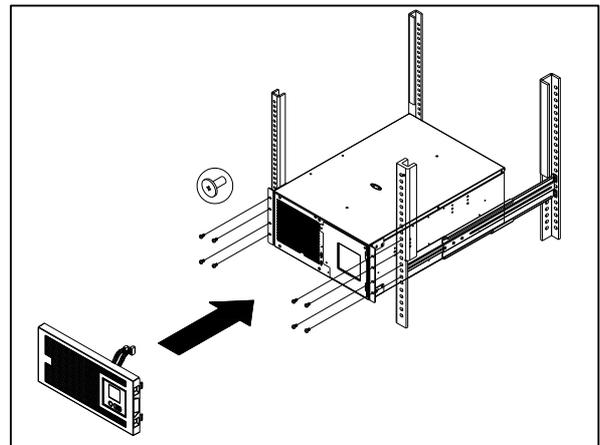
**CAUTION!** The UPS must be installed at the bottom of the rack system.
