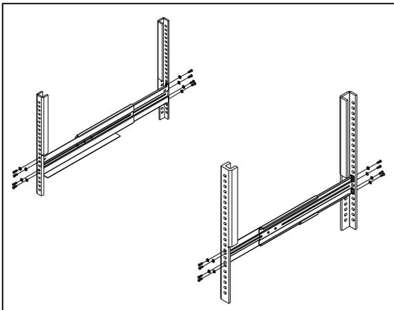
Attach the rack mount rails to your rack using fasteners that are designed for your rack system.
