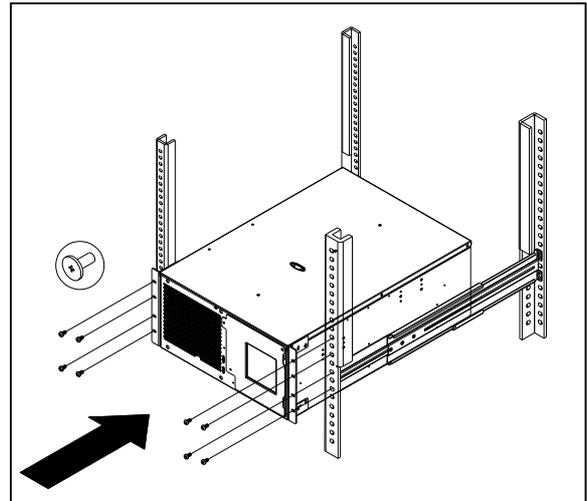
Take the rack mount rail inscribed with an "L" (Left) and attach it to the rear bracket of the Rack-mount Rail using three (3) of the six (6) Rack-mount Rail Screws. Do not fully tighten the rack mount rail screws, as the rack mount rails will need to be adjusted to fit your rack. Once complete, perform the same steps for assembling the Rack-mount Rail inscribed with an "R" (Right).
