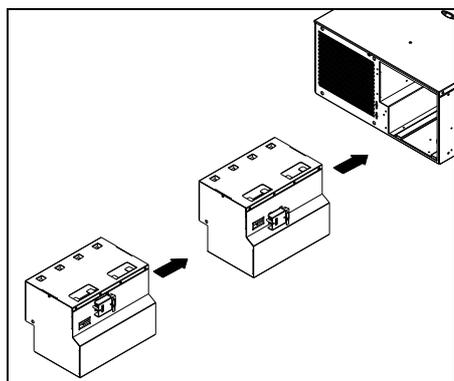
④ Put the new battery modules back into the compartment.
