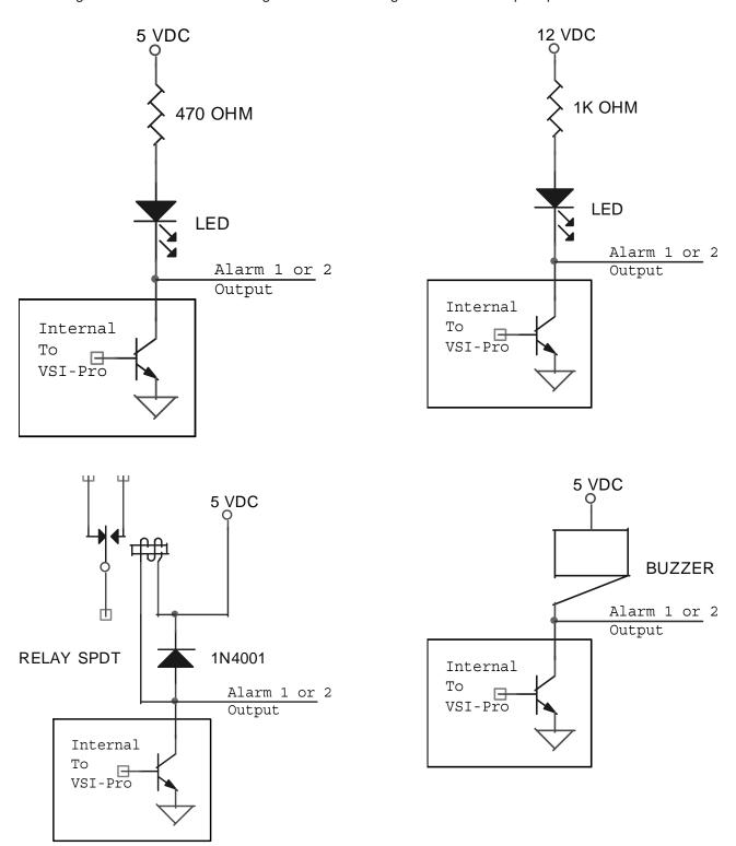
Figure 1H: Hard Alarm Output
