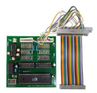
Figure 1G: TK6000/7000 PCB and Cable
