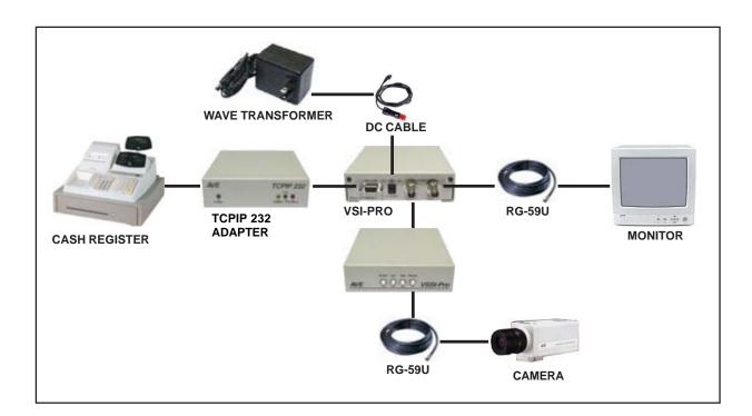
Figure 3H: VSI-Pro Connections with TCPIP 232 Adapter
