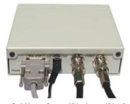
Serial Input Power Video Input Video Output
