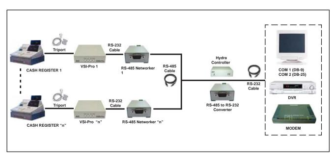
"n" means up to 64 Cash Registers / VSI-Pros / RS-485 Networkers can be connected on one RS-485 Network
