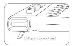
► note The USB ports on your keyboard can be used to power any USB device that consumes less than 100 mA (milliamperes), including most digital cameras, card readers, keyboards, mice, MP3 players, thumb drives and many other handheld USB devices.
