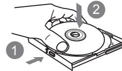
1. Press the drive release button to open the drive. Pull gently once it pops open.
