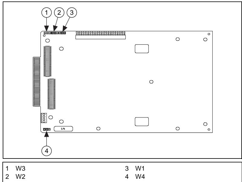
**Figure 3-1.** PXI-8170 Series I/O Board Parts Locator Diagram
