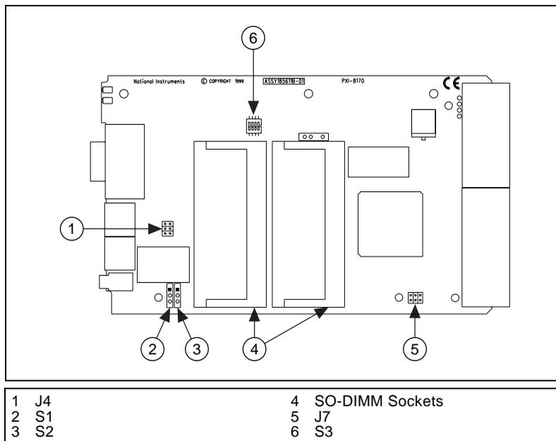
Figure 3-2. PXI-8170 Series CPU Board Parts Locator Diagram
