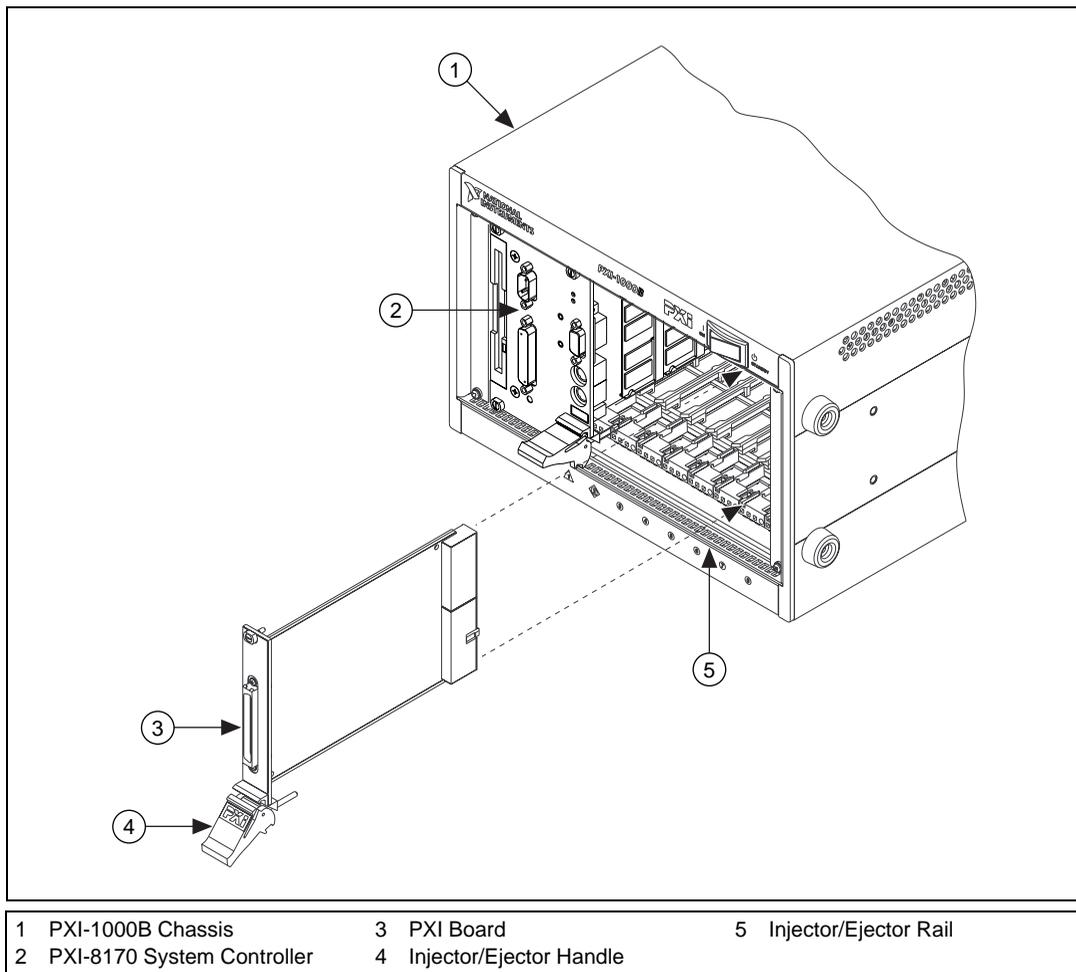
**Figure 3-3.** PXI-8170 Installed in a PXI Mainframe
