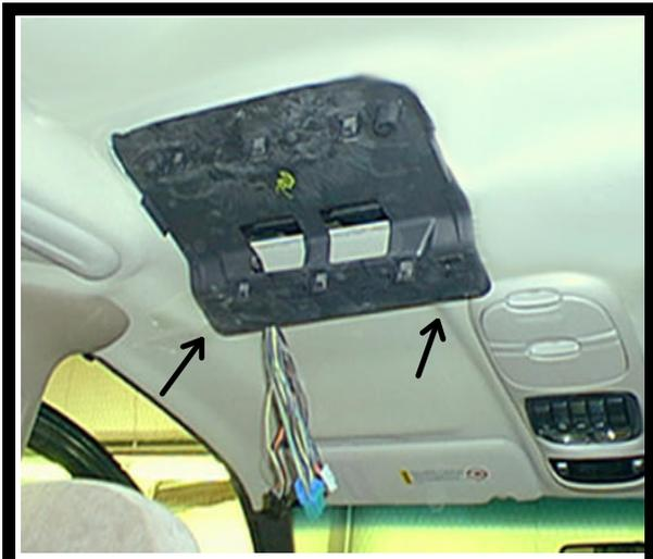
3. Remove and retain (2) two O.E.M. screws which secure plastic panel. Slide panel rearward until front edge of panel can be lowered through headliner. Slide forward and discard panel. See Figure 3.
