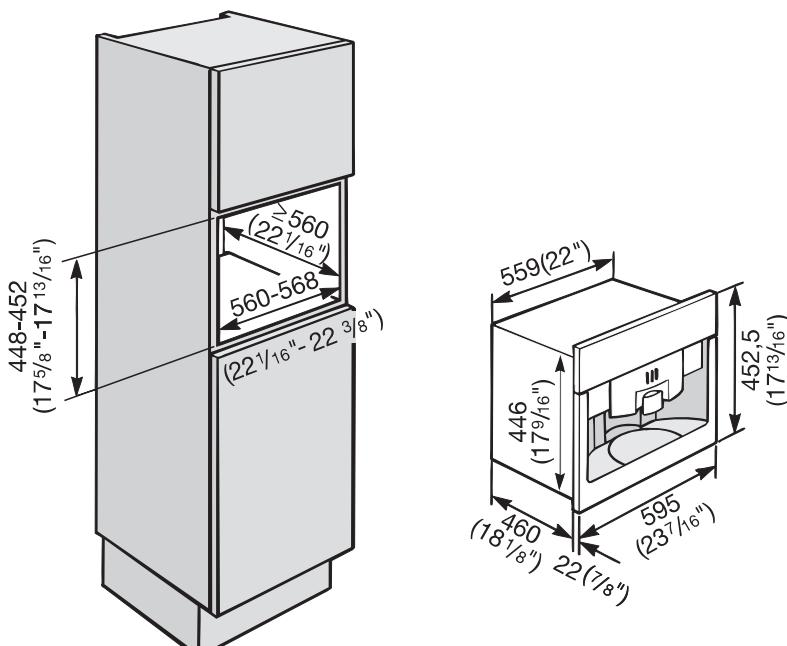
A combination with other Miele built in appliances is possible. If the machine is installed in combination with other appliances, it should be installed with a protective base between the appliance and the unit (exception: installation with a built-in plate warmer).
